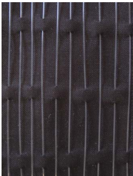
Figure 29: Picture of the black lamella with straight, inserted optical fibres
