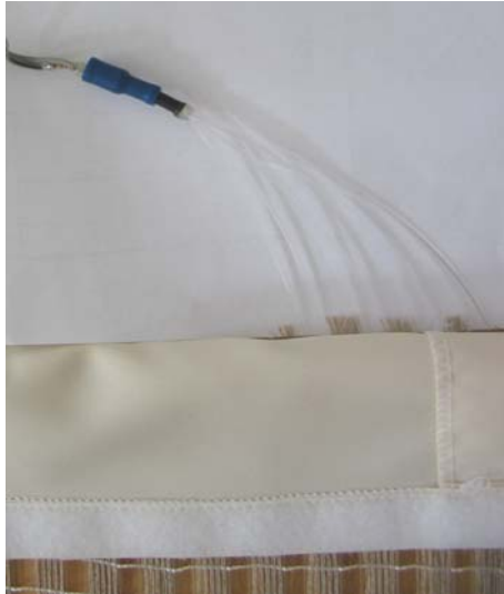
Figure 37: Connection between the optical fibres and the light emitting diodes in the Panel Curtain
