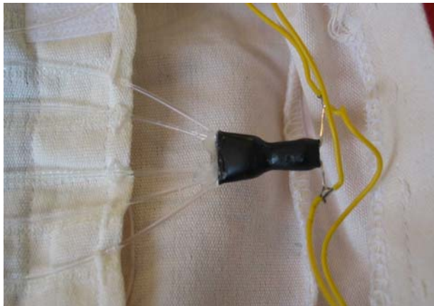
Figure 15: Picture of the connecting part between the light emitting diode and the optical fibres with the shrinking tube and hot melt adhesive
