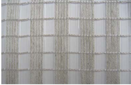
Figure 10: Warp knitted fabric with optical fibres inserted as weft threads
