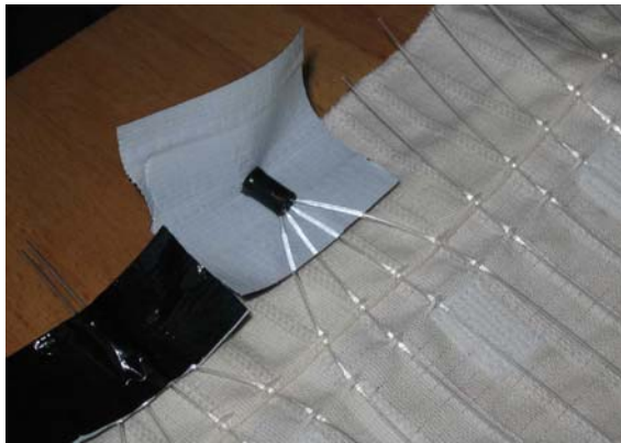
Figure 19: Connecting part, made of black adhesive tape, between the light emitting diode and four optical fibres. The diode is covered separately in black adhesive tape. Also on the picture are two floats in a short distance for getting the optical fibres parallel.
