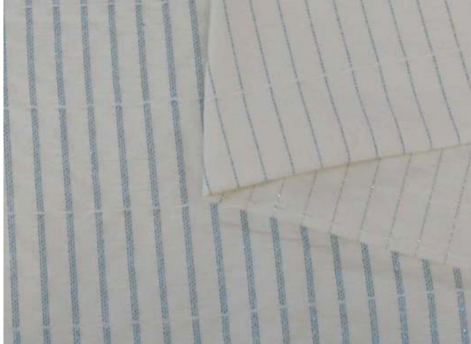
Figure 5: Front side weave with floats for fastening the optical fibres
