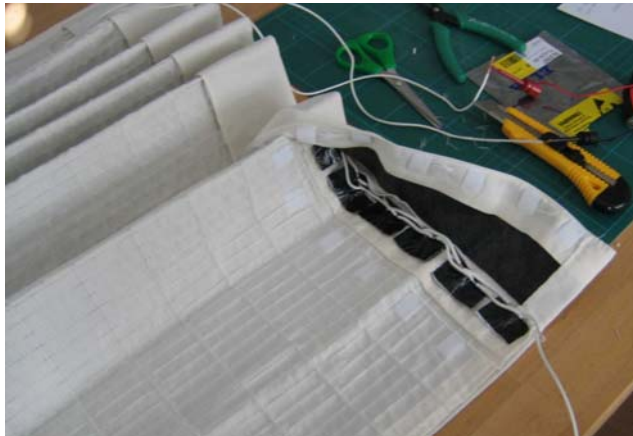
Figure 21: Connecting elements between optical fibres and light emitting diode under the overlap on the side. The white cables connect the light emitting diodes.
