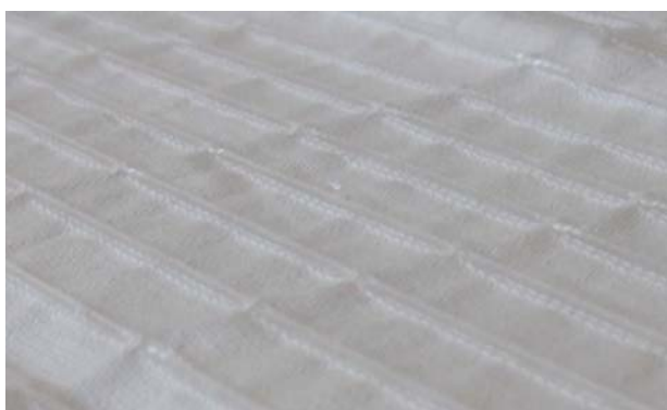
Figure 11: Inserted optical fibres under the floats
