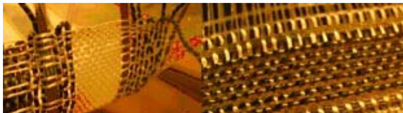
The conductive materials as heat elements are integrated directly into the fabric during weaving.
