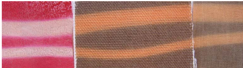
Conductive heat transmitting threads sandwiched together with fabric.
