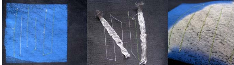
The pictures show a blue thermochromical print made on conductive fabric which has metallic wirers stitched on the backside.
