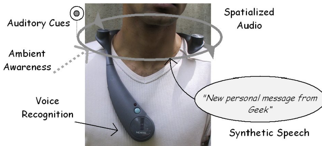
Figure 2.2 The SoundBeam Neckset used as an interface for the Nomadic Radio. (Sawhney and Schmandt, 1999, p. 2)
