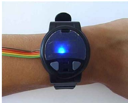
Figure 6: The wrist-watch device is here signaling that the "blue child" is in trouble.
