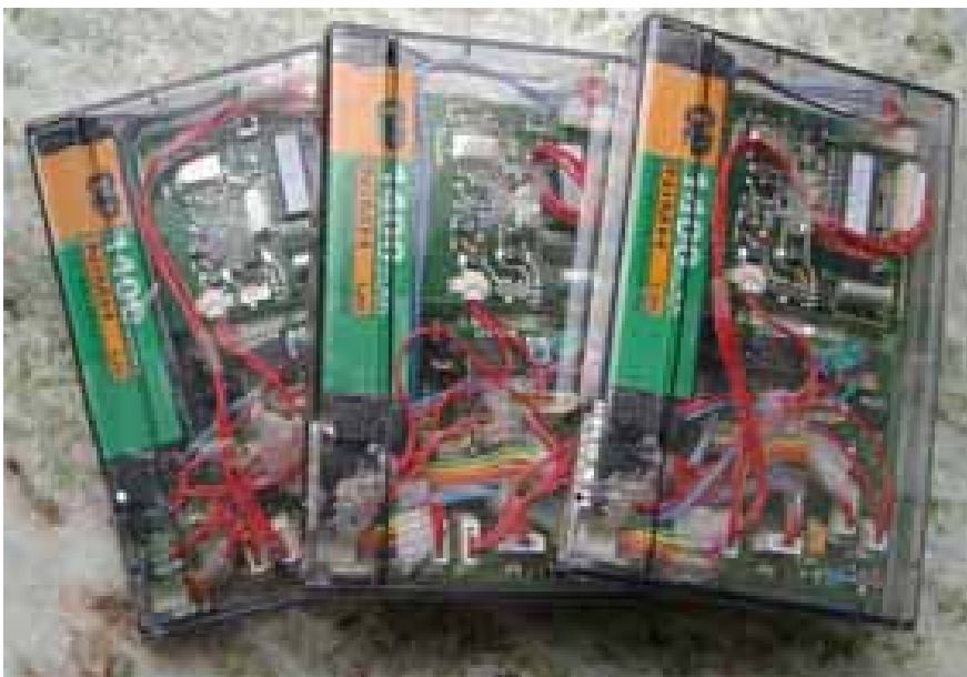
Figure 5: Three Smart-Its boxes ready for use. The transparency of the boxes is necessary as the boards contain various visual actuators.
