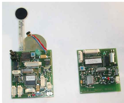
Figure 4: The Smart-Its boards, to the left the sensor board and to the right the RF-board.
