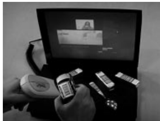
Figure 1: Users manipulate various objects to view “memories” in the form of multimedia clips, which when taken together will form a narrative
