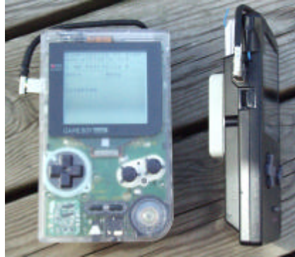
Fig. 2. Picture showing the Generalised Hummingbirds, i.e., GameBoys fitted with radio transceivers.
