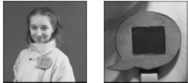
Figure 1 & 2: The BubbleBadge display, connected to a hidden wearable computer
