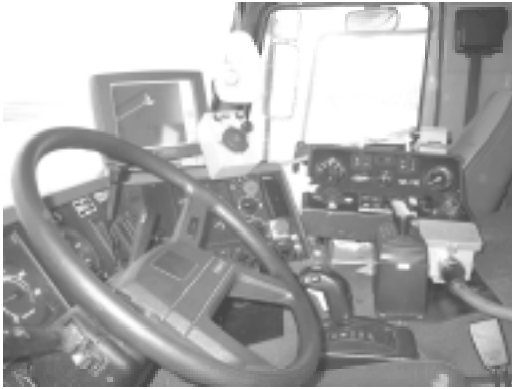
Figure 2. The inside of one of the snow vehicles. The SnowCard display is in the upper left corner of the picture. The small radio receiver is hanging down from the ceiling of the vehicle, and is visible in the top middle of the picture.
